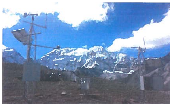
Figure 7: Hydrological & Meteorological stations with communication system installed for Imja Lake
